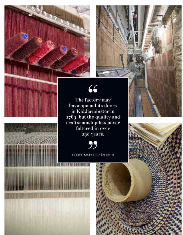
Clockwise from top left: Yarn delivery to the loom, an Axminster loom, a finished Axminster carpet on the roll and backing yarn.
